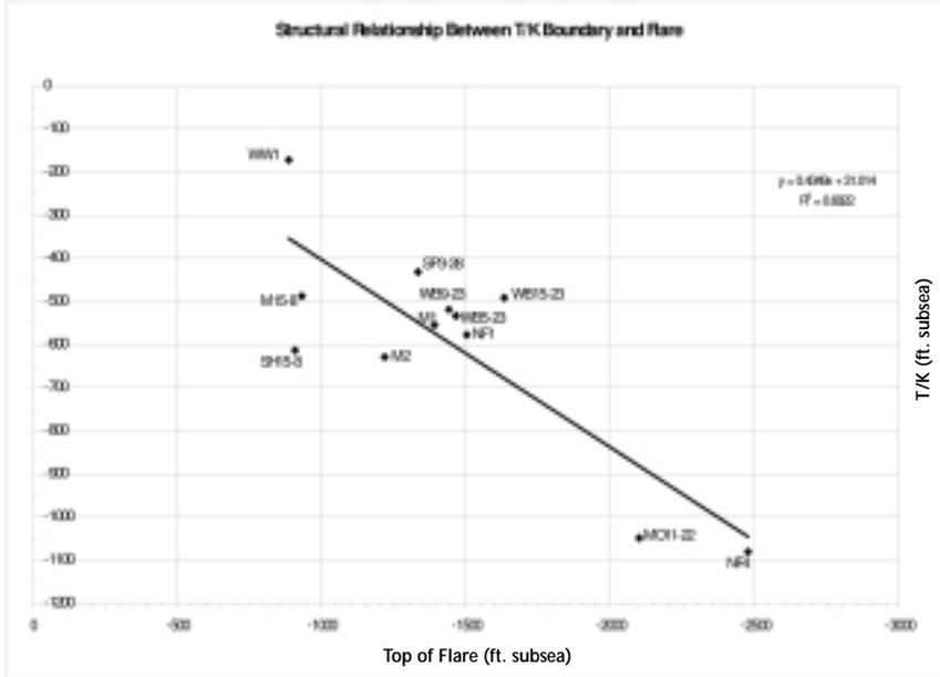
Figure 4.6. Subsea top of flare (Lance Formation) plotted against Subsea depth of Tertiary-Cretaceous boundary. Source: Ultra Petroleum.
