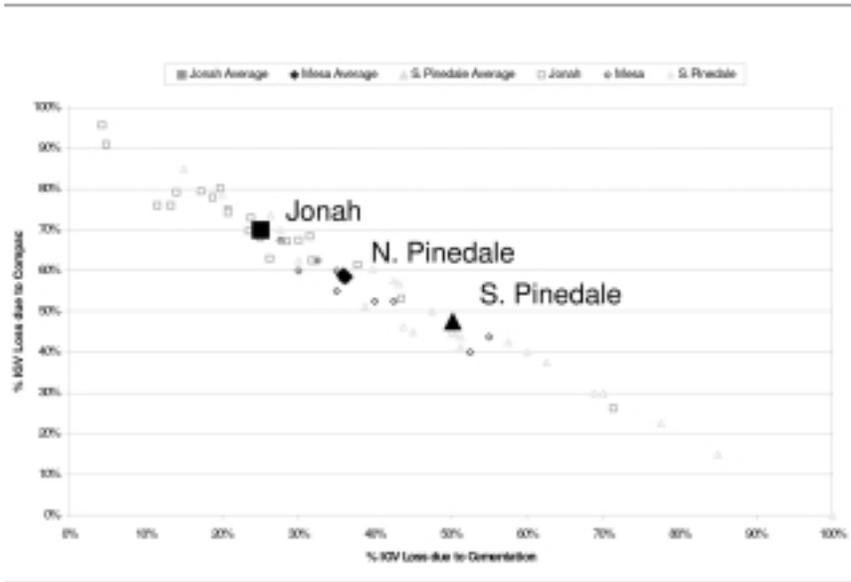
Figure 4.8. Loss of intergranular pore volume by compaction versus by cementation for Pinedale and Jonah fields. Source: Ultra Petroleum.
