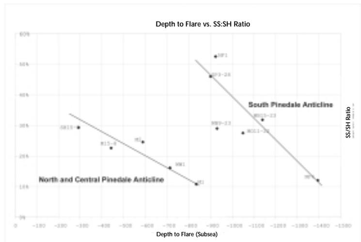
Figure 4.7. Subsea top of flare plotted against sandstone/shale ratio (in %). Source: Ultra Petroleum.
