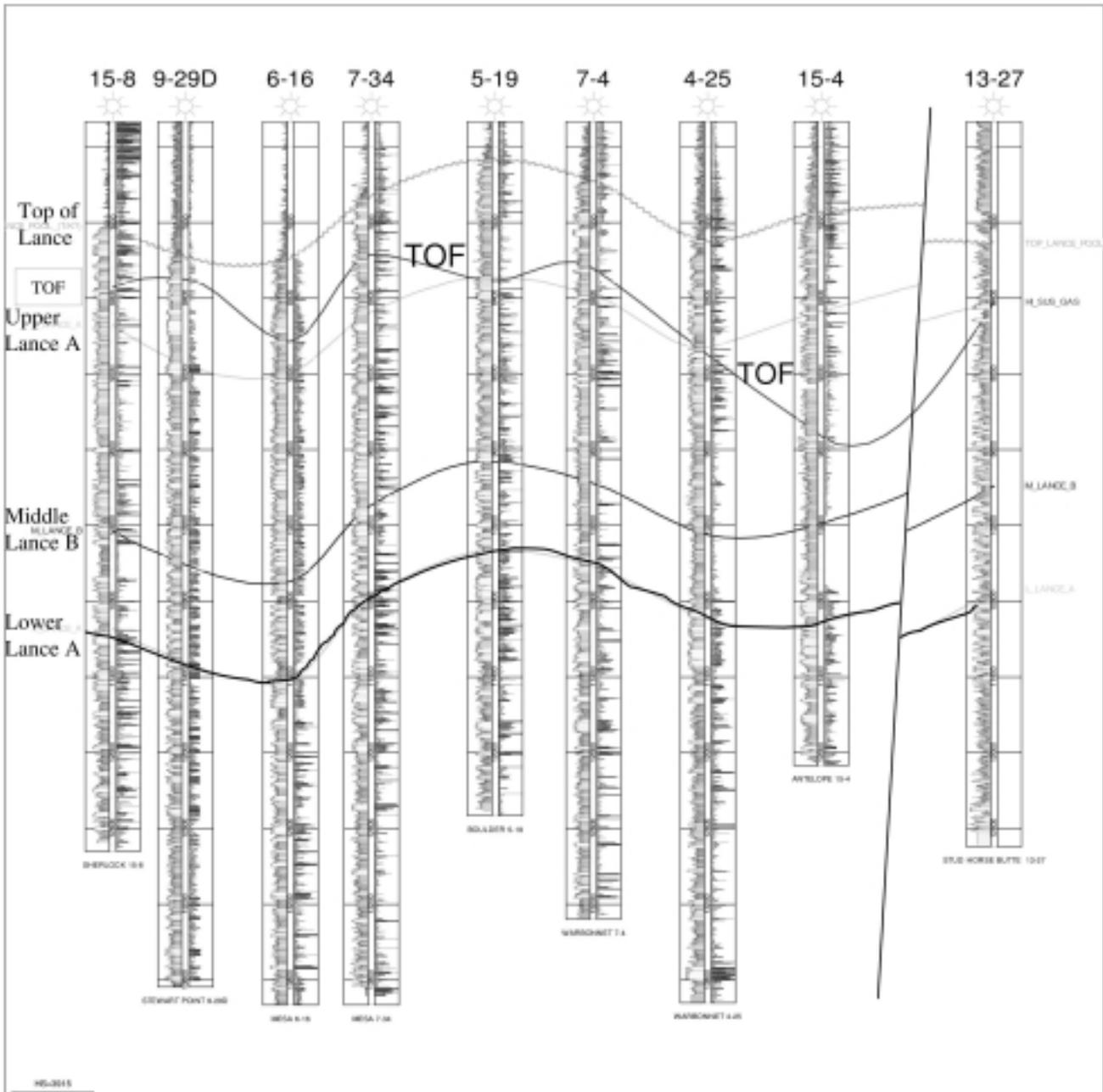
Figure 4.5. North-south structural (strike) cross section, Pinedale Anticline to Jonah Field. Section shows that top-of-flare does not accord with stratigraphy along strike of anticline. Source: Ultra Petroleum.
