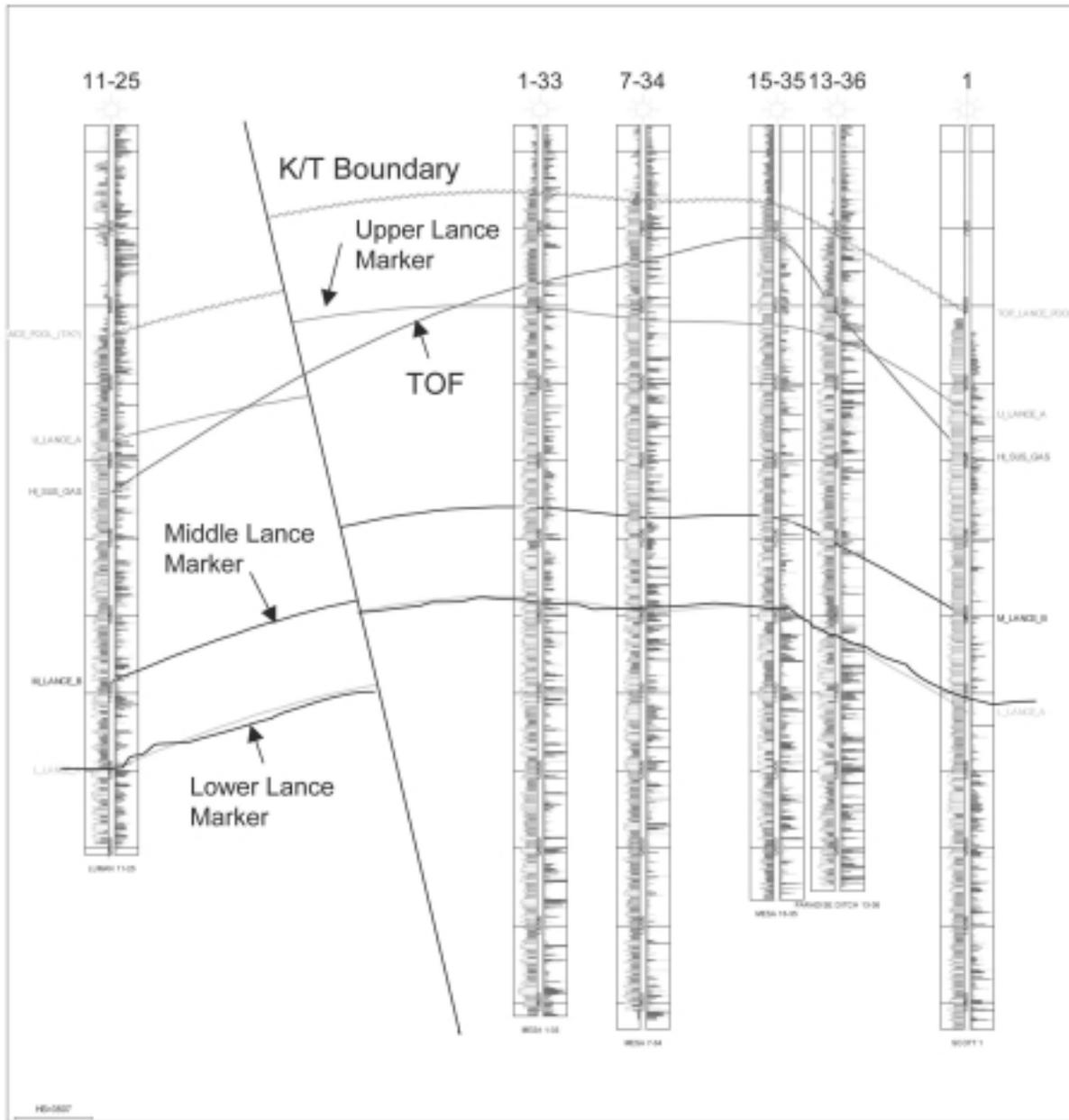
Figure 4.4. West-east structural (dip) cross section, northern Pinedale Anticline (Mesa area), showing selected stratigraphic markers and top of sustained gas (top of flare = TOF). Section is hung from 7800-ft depth line. Source: Ultra Petroleum.
