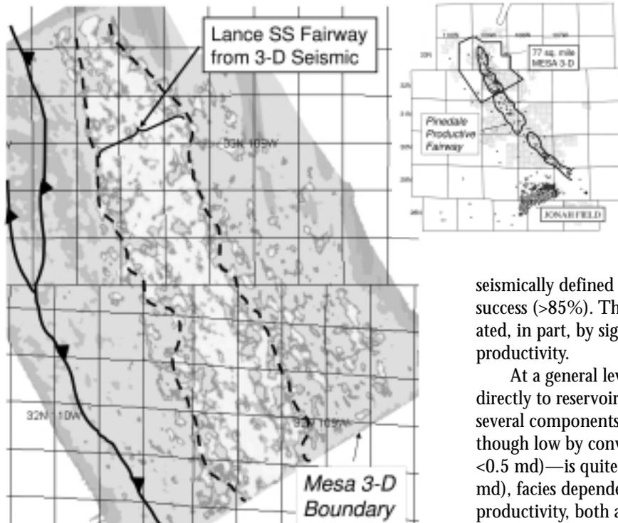
Figure 4.1. Outline of Lance Sand fairway, northern Pinedale Anticline (Mesa area), based on attribute analysis from 3-D seismic data. Adapted from Ultra Petroleum.
