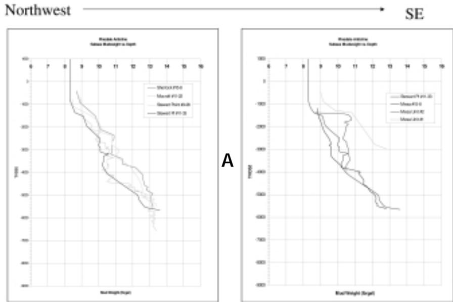
Figure 4.10. Mud weight profiles for wells in Pinedale Field. A) Stewart Point – Mesa areas; B) New Fork – Warbonnet areas. Source: Ultra Petroleum.
