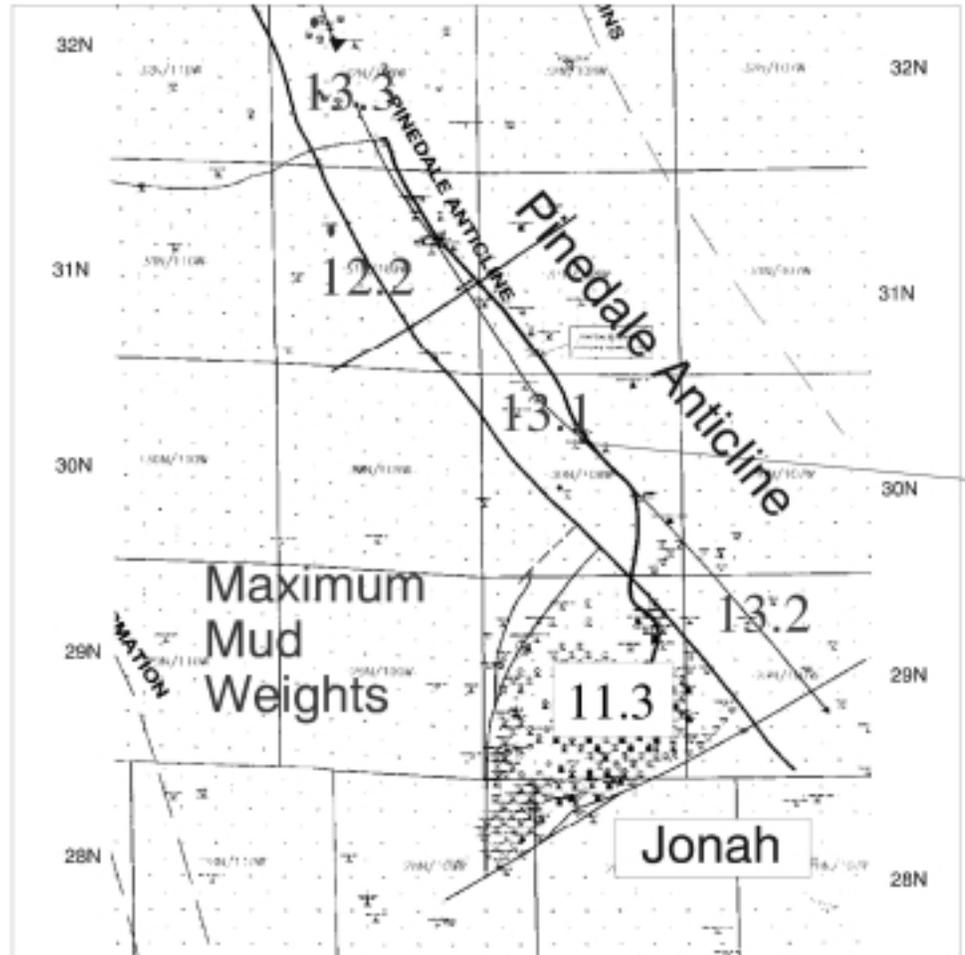
Figure 4.11. Maximum mud weights within Lance Formation, for different portions of Pinedale Anticline and Jonah Field. Source: Ultra Petroleum.
