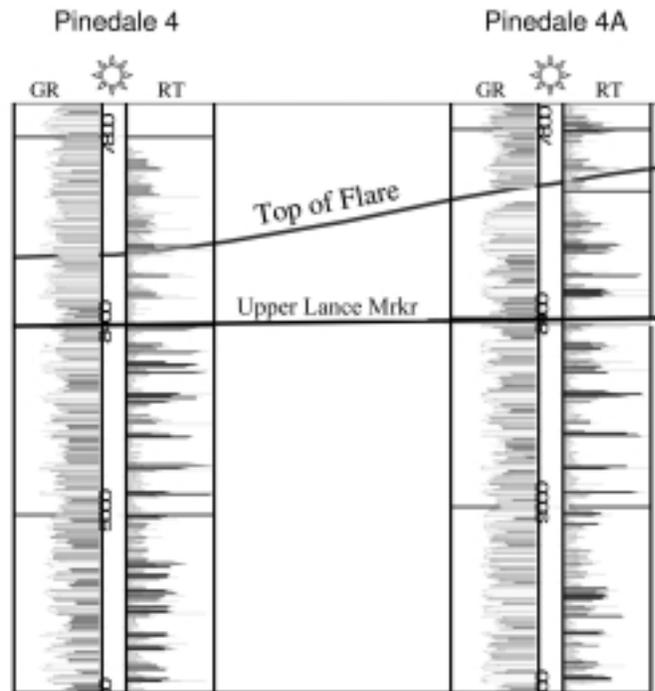
Figure 4.3. Enlargement of Figure 4.2 (part), including productive portion of upper Lance, below top of flare. Lateral heterogeneity shown by these closely spaced wells (~50 ft horizontal separation) suggests difficulty of mapping individual reservoir zones, either through log or seismic data. Such heterogeneity also implies the need for close spacing to adequately drain the Lance. Data courtesy Ultra Petroleum.
