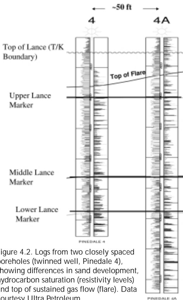
Figure 4.2. Logs from two closely spaced boreholes (twinned well, Pinedale 4), showing differences in sand development, hydrocarbon saturation (resistivity levels) and top of sustained gas flow (flare). Data courtesy Ultra Petroleum.
