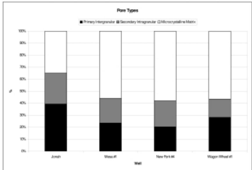
Figure 4.9. Pore type differentiation for different areas, Jonah-Pinedale fields. Source: Ultra Petroleum.
